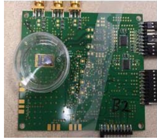
Fig. 8. Test setup for impedance mapping.
